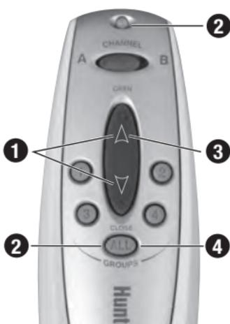
4. Press the ALL button to save the stop. The Indicator Light stops flashing.
