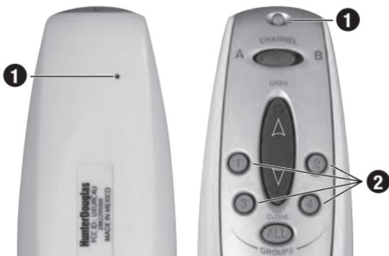
2. While the Indicator Light is flashing green, press the group button for the group to which you plan to assign the window covering.
