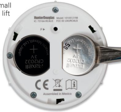
5. Insert new batteries, making sure each is snug.
