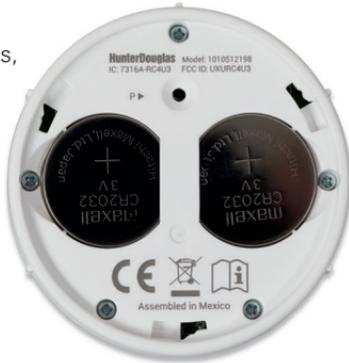
6. Align and replace the back cover onto the backside of the remote module.
