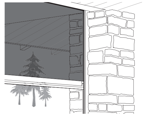
Built-in Oasis 2900 with recessed sidetrack in masonry columns.
