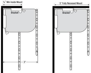
Attach the installation/extension brackets using the screws provided.
