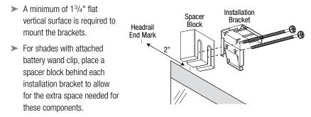
> The top of the installation brackets should be at the desired shade height.
