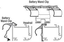
**CAUTION:** Be sure the power cable does not become pinched by the brackets or headrail during installation; damage or overheating of components could result.
