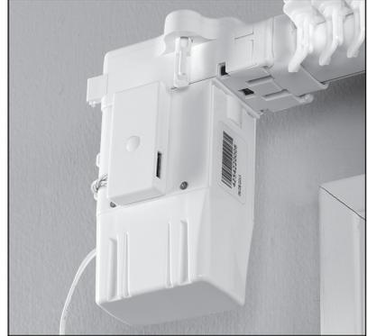
**IMPORTANT:** If snapping the motor onto the drive assembly seems difficult, grasp the lead carrier and pull the carriers slightly away from the motor, as shown at right. The motor should now snap in easily.
