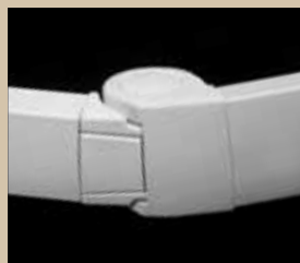
Cables hidden while arm extended
